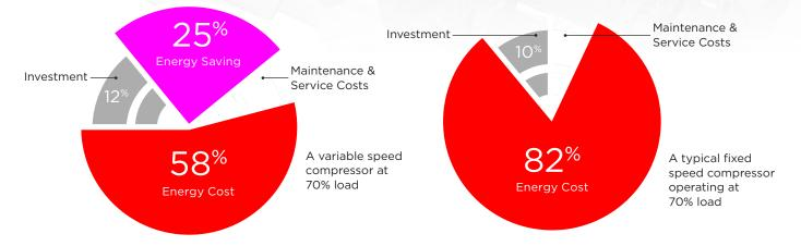
Using a variable speed compressor can easily save 25% energy by using just the right amount of energy required to do the job and no more.
